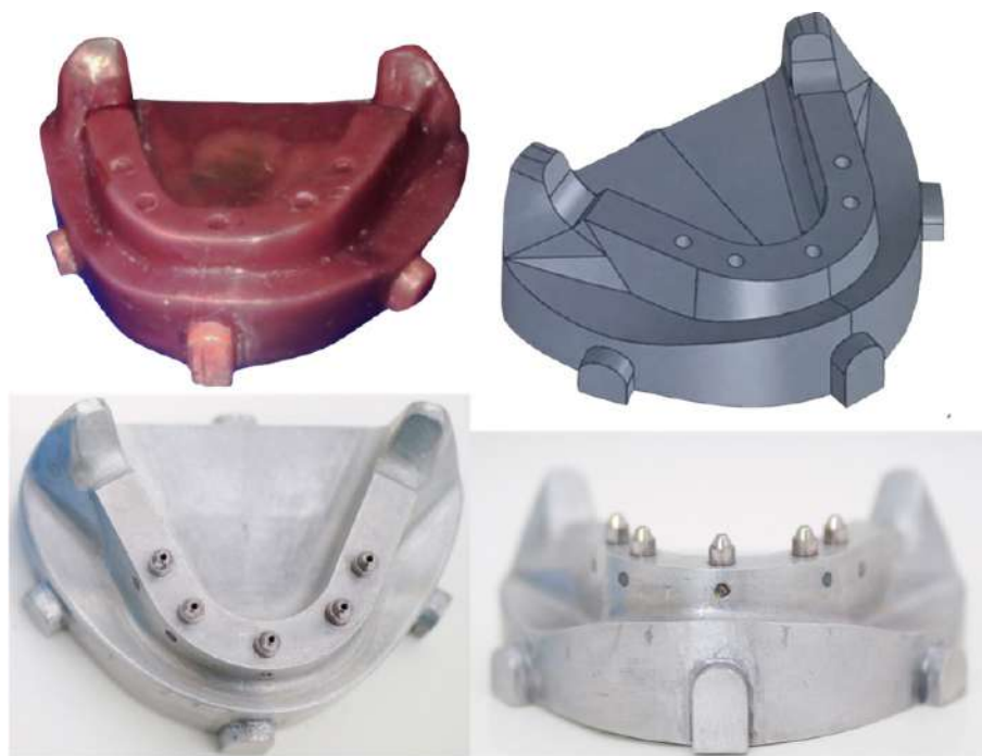
Figure 2. Pattern model scheme and distribution of analogs.
